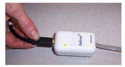
3. Plug the other end of the USB connector into the back of the Scan Station.
